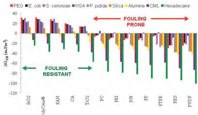
Figure 5. Plots of (top) free energy of cohesion or hydrophilicity for common polymeric and ceramic membrane materials and (bottom) free energy of adhesion or fouling propensity for polymeric and ceramic membrane materials along with a wide range of organic, microbial and inorganic fouling materials
