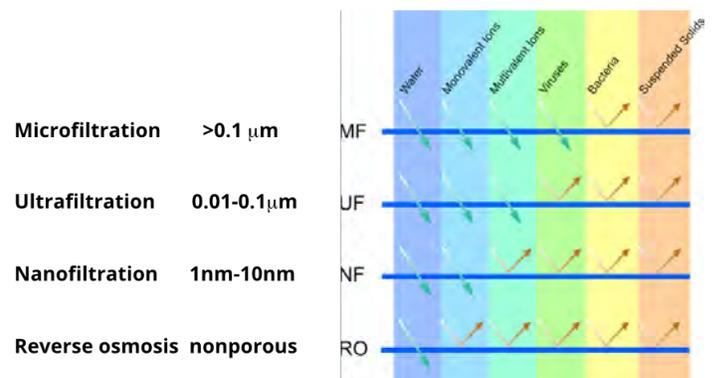
Figure 1. The membrane filtration spectrum showing all forms of pressure-driven membrane processes by pore size, typical designation and classes of substances removed.
