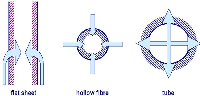
Figure 4. Different filtration flow regimes employed in different membrane module form factors.
